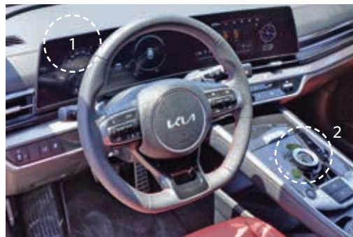
The (1) dual 12.3-inch curved display - one for instruments and the other for the central touchscreen panel - and (2) shift-by-wire rotary dial are now standard across all trims
