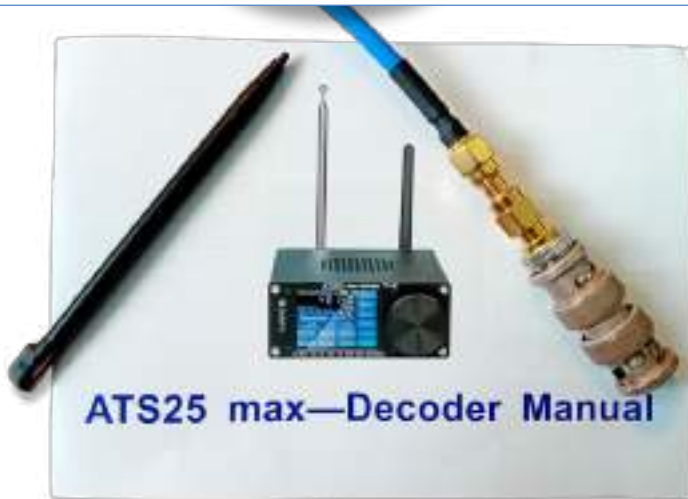
Figure 2: My makeshift SMA-to-BNC adapter (in two steps but 50 \Omega throughout), the indispensable stylus (left) and the printed manual.
