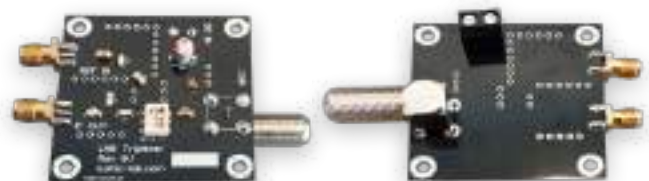
Figure 8: The triplexer for reference frequency and IF signal separation and supply voltage injection. On the back side (right), the F connector for the LNB and the input voltage screw-terminal block are located.
