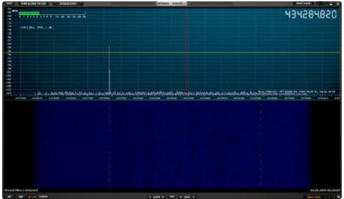
Figure 12: The received IF signal's SDRuno spectrum display, with clearly visible frequency hops spaced 1 MHz apart.
