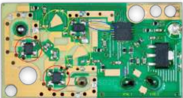
Figure 3: Top view of the LNB's PCB. Please refer to the text for identification of the various components.
