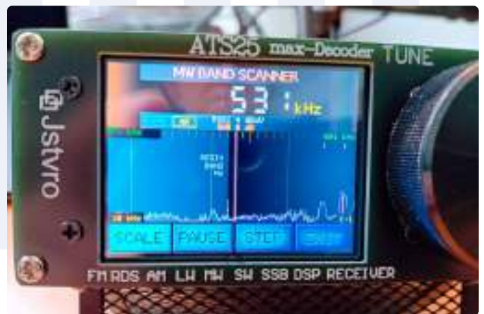
Figure 1: Scanning the MW band for activity using the built-in spectrum analyzer. Not a lot to hear at daytime but come again near dusk and the party starts.
