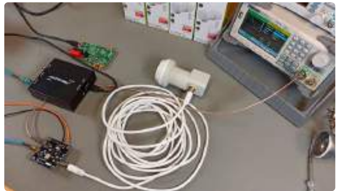
Figure 10: Test setup with a signal generator, triplexer, SDR receiver and ADF4351 used as third-harmonic X-band signal generator.
