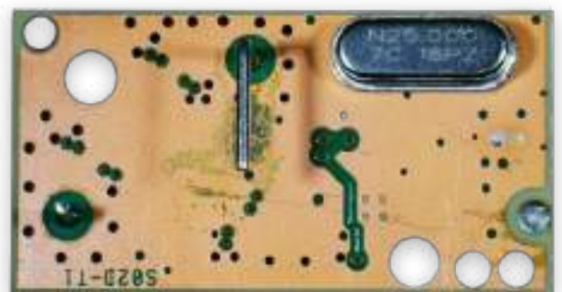
Figure 4: Bottom view of the PCB, with the 25 MHz reference crystal in the top-right corner.
