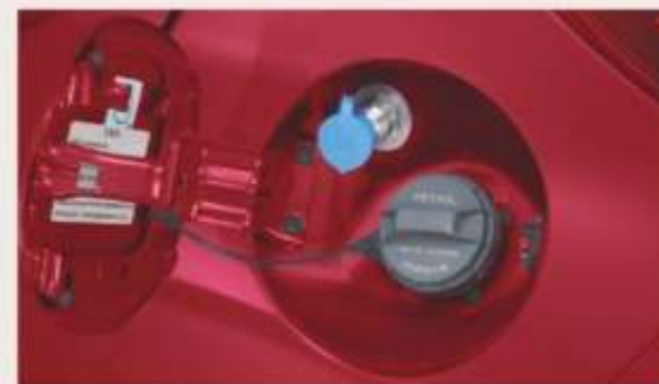
Convenient CNG filling with fast refuelling nozzle (near petrol filling area)
